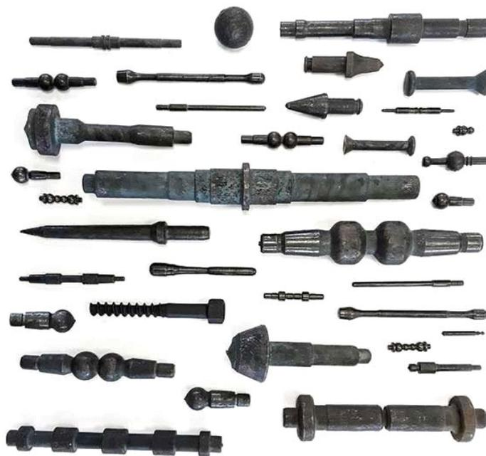
**Figure 1** - Examples of parts produced by cross wedge rolling [4].
